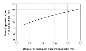
Fig. 4. Free fall velocity of absorption slurry droplets
