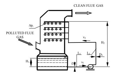
Fig. 1. Circulation of absorption slurry in the system: slurry reservoir - the highest level of slurry spraying in absorber
