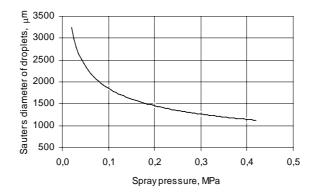
Fig. 3. Average Sauter's diameter of droplets versus absorption slurry spraying pressure
