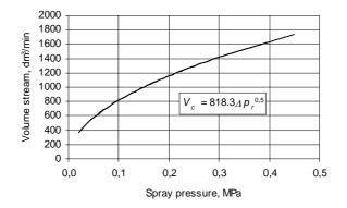
Fig. 2. Characteristic curve of work of eccentric atomizer of CaCO<sub>3</sub> slurry
