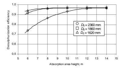
Fig. 5. Desulphurization efficiency versus height of absorption zone in vertical spray absorber and diameter of absorption slurry droplets ( $L/G = 12 \text{ dm}^3/\text{m}^3$ )
