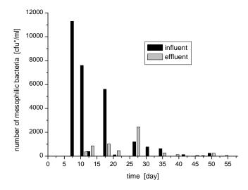
Fig. 9. Total mesophilic bacteria changes in influent and effluent
