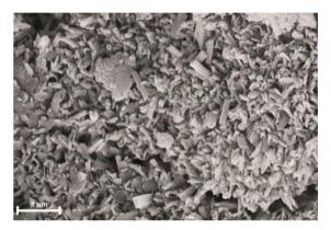
Fig. 1. SEM photo of layered-tubular structure of raw halloyiste from Dunino deposit
