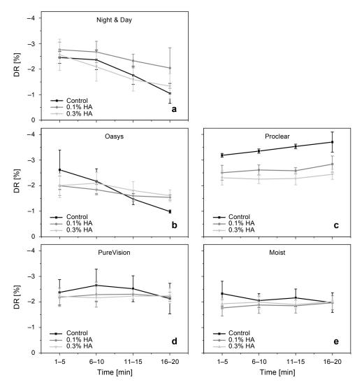
Fig. 4. Mean dehydration rate (DR) at 5 min intervals for the first 20 min: Night & Day (**a**), Oasys (**b**), Proclear (**c**), PureVision (**d**), and Moist (**e**). Vertical bars present standard deviation.
