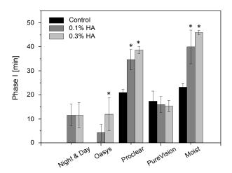
Fig. 2. Comparison of phase I of dehydration among three groups: control lenses without any solution (black bars), lenses soaked in 0.1% HA (grey bars) and to 0.3% HA (light-grey bars). Phase I was not observed in case of control Night & Day and Oasys lenses. \* - p < 0.05 ANOVA test for the difference between control group and HA solution.
