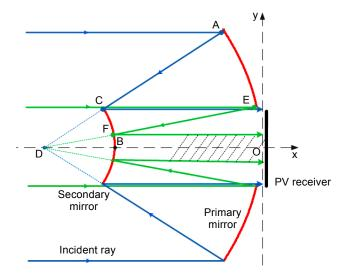
Fig. 1. Structure of Cassegrain-type solar concentration system.
