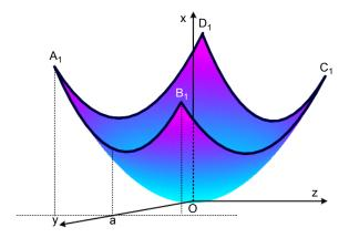
Fig. 2. Square cross-section of a rotating parabolic reflector.
