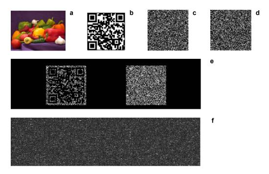
Fig. 3. The original color image (a); the corresponding QR code (b); the real part of encryption key r(x, y) (c); the real part of encryption key k(x, y) (d); the joint input image for JTC (e); the encrypted result (f).
