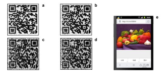
Fig. 4. The decryption QR code (**a**); the decrypted QR code corrupted by zero-mean speckle noise with a variance of 0.1 (**b**); the decrypted QR code corrupted by zero-mean additive speckle noise with a variance of 0.5 (**c**); the decrypted QR code corrupted by zero-mean additive speckle noise with a variance of 0.6 (**d**); the outcome obtained by scanning  $\mathbf{a}$ - $\mathbf{d}$  with a smartphone (**e**).
