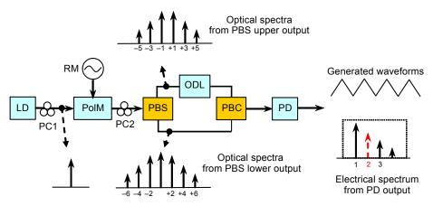
Fig. 1. Schematic diagram of the proposed triangular waveform generation system. LD – laser diode, PolM – polarization modulator, PBS – polarization beam splitter, PBC – polarization beam combiner, PC – polarization controller, ODL – tunable optical delay line, PD – photodetector.
