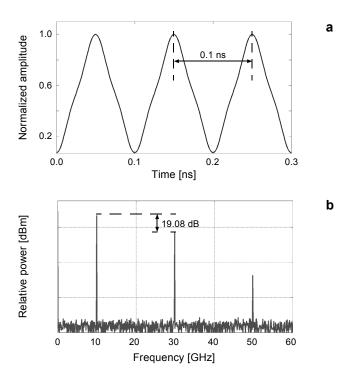
Fig. 4. The generated triangular waveform (a) and its spectrum (at the repetition rate of 10 GHz) (b).
