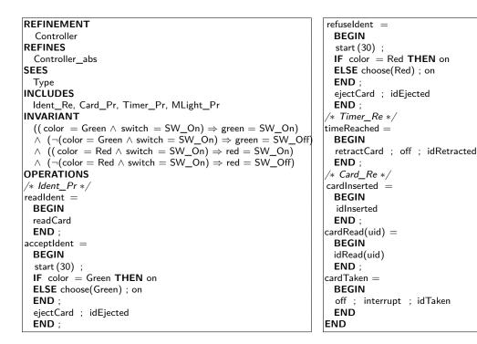
Figure 15. B Model of the component Controller
