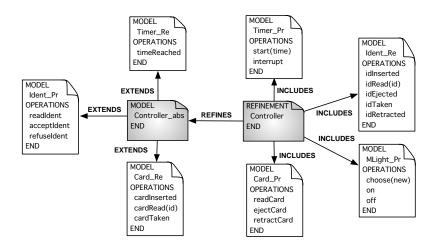
Figure 14. B architecture of the component Controller
