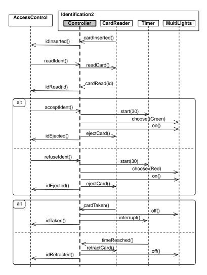
Figure 13. Sequence diagram for the Identification2 component
