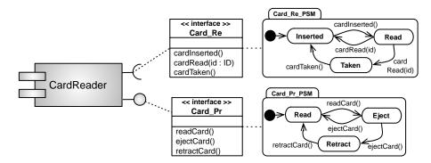
Figure 9. Component CardReader and its interfaces Card\_Pr and Card\_Re
