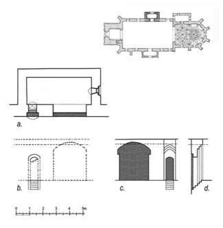
Fig. 4. Preliminary interpretation of the openings in the upper floor of north porch: a) throw on the level of discovered openings,b) view form the church side, c) view form the porch side,d) cross-section on the level of smaller opening (drawn by M.R. Gogolin, J.M. Arszyńska)
