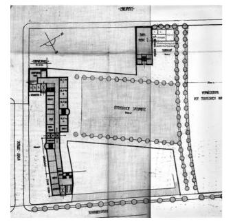
Fig. 2. Situational plan of the folk school building and the object with gymnasiums along with the marked planned area of the extension of the Higher School of Technology on the west side of Norwida Street; project: Max Berg, October 10, 1913 [2, p. 271 (fragment)]
