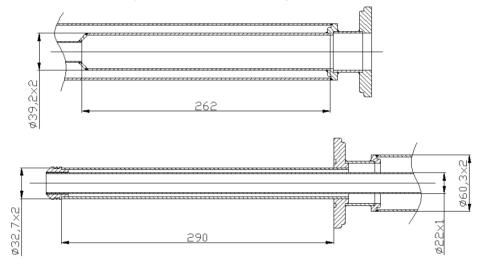
Figure 3. Dimensions of the bayonet connector
