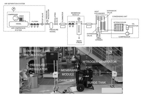
Figure 2. Test stand of air separation system
