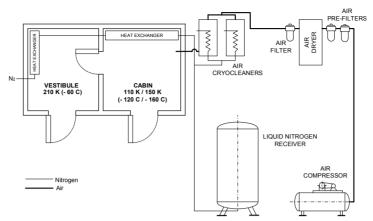
Figure 2. Structure of the cryochamber system
