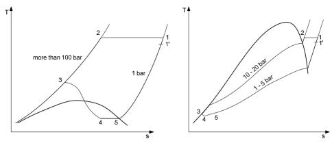
Figure 2. Thermodynamic processes for pure gas cycle on T-s diagram, thermodynamic processes for gas mixture cycle on T-s diagram
