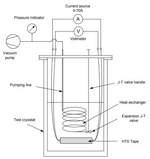
Figure 4. Scheme of test stand
