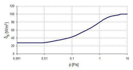
Figure 4. Heat flux by the residual gas as a function of pressure
