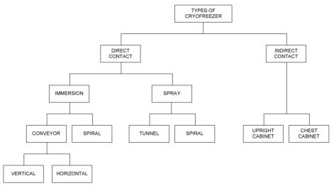
Figure 1. The classification of cryofreezers
