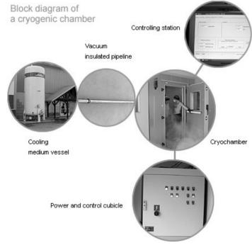
Figure 5. Block diagram of a cryochamber [4]
