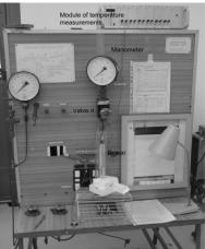
Figure 3. Test stand of Joule-Thomson liquefier
