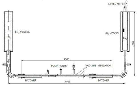
Figure 1. Test stand for estimation of heat transport to the cryogenic transfer line.
