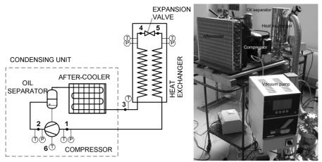
Figure 3. Test stand of J-T refrigerator
