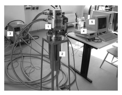
Figure 2. Gifford-McMahon refrigerator performance test stand: 1 – two stage Gifford-McMahon cryocooler, 2 – vacuum vessel, 3 – helium compressor, 4 – cryocooler coldhead temperature controler, 5 – DAQ system
