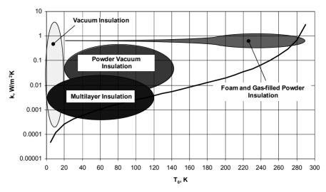
Figure 2. The classification of cryogenic thermal insulations
