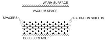
Figure 1. Structure of multilayer insulation (MLI)
