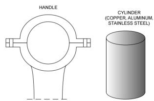
Figure 2. Test stand for the shrink-fitting technique.
