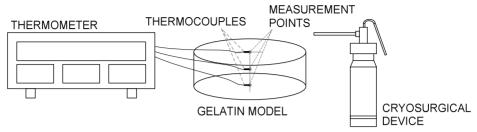
Figure6. The test stand for the cryosurgical process simulation (contact and spray method).
