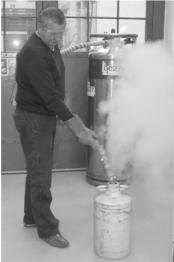
Figure 1. The technician fills Dewar with liquid nitrogen
