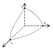
Figure 1. Critical surface superconducting phase diagram
