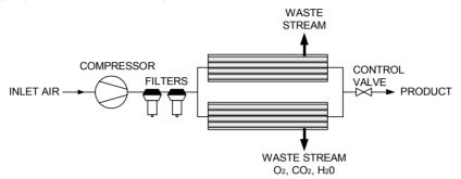
Figure 1. Polymeric membrane air separation system
