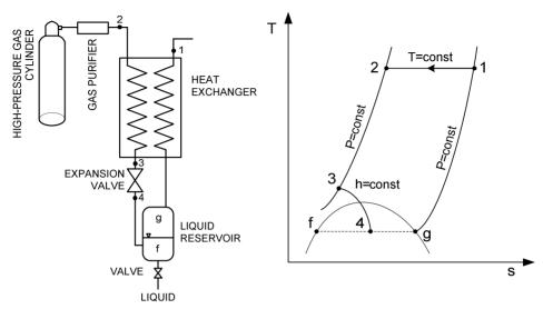
Figure 2. Joule-Thomson liquefier, thermodynamic processes on T-s diagram
