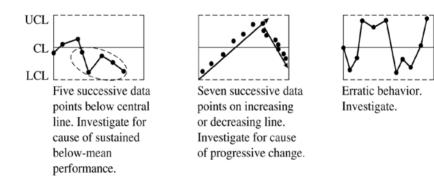
Fig. 17. Examples of process performance measurement by Six-Sigma concept for SPC method/technique.
