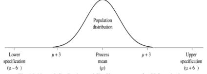
Fig. 15. Normal distribution and Six-Sigma concept for SPC method.
