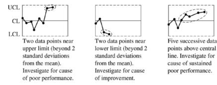
Fig. 16. Examples of process performance measurement by Six-Sigma concept for SPC method.
