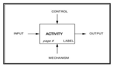
Fig. 36. IDEF0 model syntax - function box and interface arrows (ICOM Box). Source: www.kbsi.com
