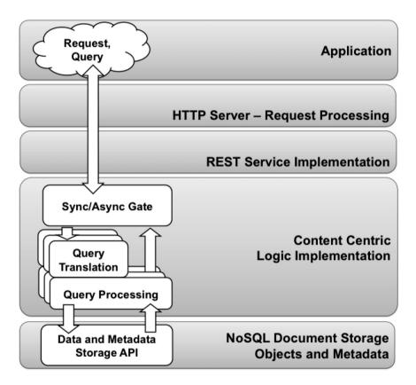
Figure 3. Content-centric service implementation: runtime view
