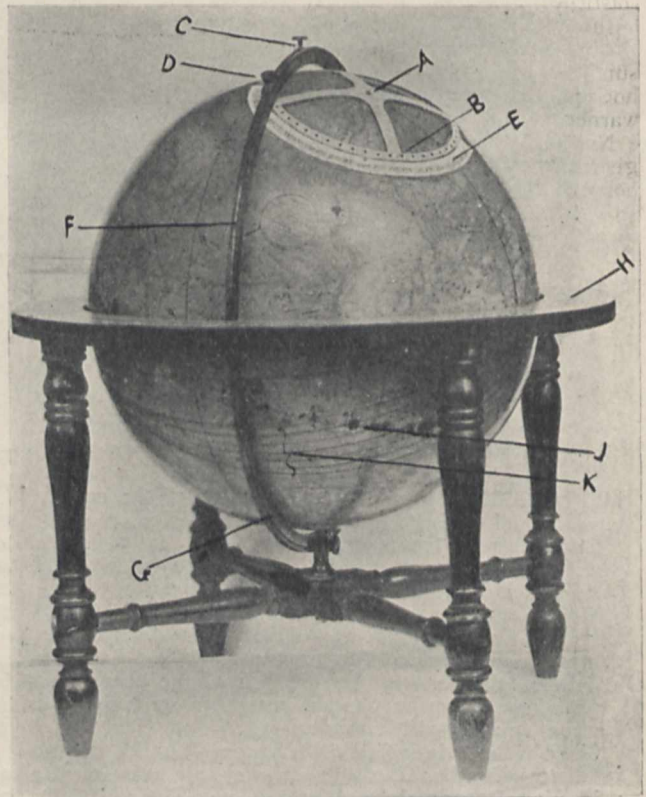
FIG. 28.—The Precessional Globe. A, Pole of ecliptic; B, brass circle, with holes on positions of celestial poles at different epochs; C, screw pivot for N. pole of ecliptic; D, screw pivot for N. celestial pole at different epochs; E, scale of years denoting position of celestial pole at definite epochs (set for 1364 B.C.); F-G, brass meridian; H, H, H, H, wooden horizon; J, ecliptic; K, celestial equators drawn for different epochs.
