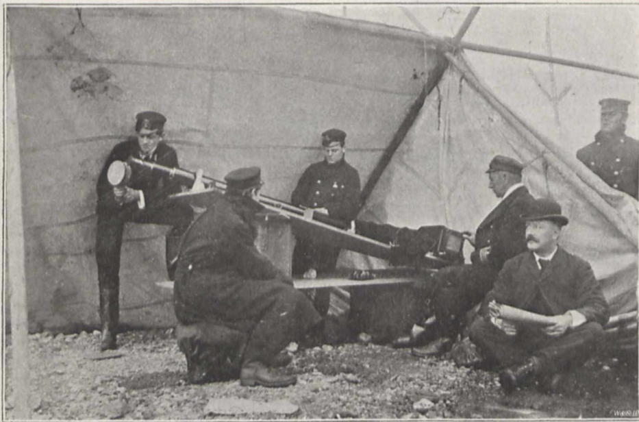
FIG. 7.—The Integrating Spectroscopic Camera.
