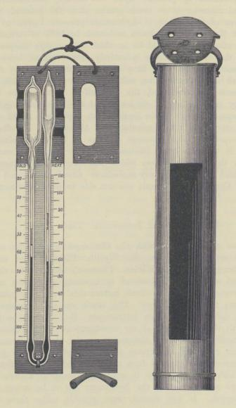
first invented form of protected thermometer, which (so far as I know) was introduced by Sir William Thomson<sup>1</sup>, is simply that the bulb only is protected, the stem being
