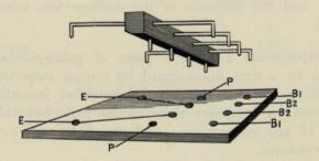
quadrants of the electrometer, P with the electrodes,  $B_1$  with the decomposing battery, and  $B_2$  with the auxiliary (or charging) battery. Also metallic connection, as indicated in the sketch, is permanently established between the two central holes and the holes connected with the electrometer.
