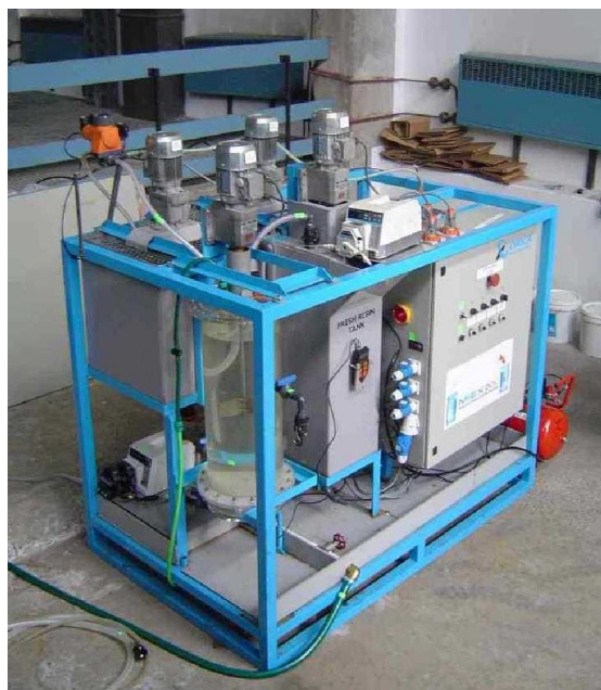
Fig. 1. MIEX ® DOC pilot plant
