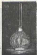
FIG. 12.—Globular spark produced over distilled water by an electric current of high tension.
