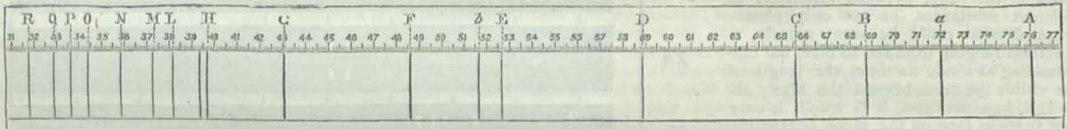
FIG. 6.—Wave-length solar spectrum showing the lines (from L to R) the positions of which have been determined by Mascart, and showing also how short the ultra-violet spectrum of the sun is as compared with that of the chemical elements.
