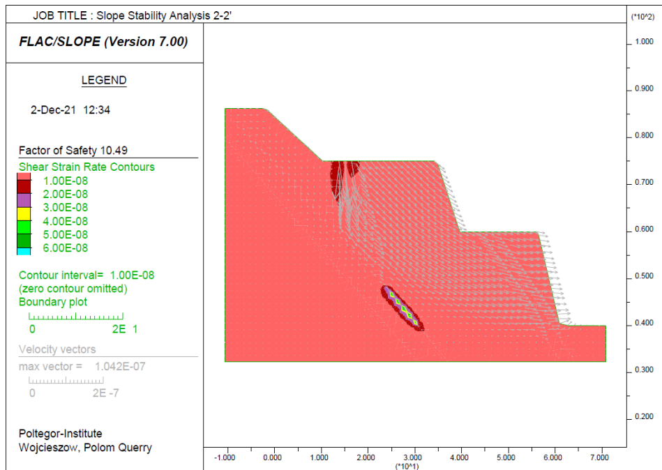
Fig. 11. Slope stability analysis, shear stresses, factor of safety F_{os} = 10.49
