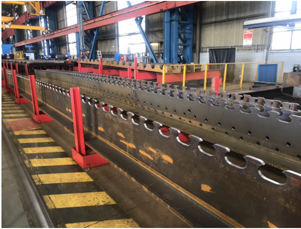
Figure 10: Steel T-sections produced in Luxembourg (picture: ArcelorMittal).
