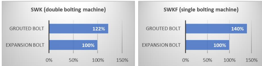
Fig. 1. Comparing the cost of grouted and expansion bolting at Lubin Mine in Q1 2020 (based on the data from the Standards Department of KGHM Polska Miedź S.A. “Lubin” Mine)
