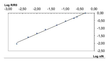
Fig. 2. The analysis of the surface density of the probability of epicenter occurrence. Fractal dimension of the distribution is D = 1,18 (Idziak,1996)
