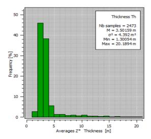
Fig. 20. Histogram of averages Z<sup>\*</sup> of thickness [m] distribution in enclosed Cu ore deposit; the block R-1, "Rudna" mine; skewness  $g_1 = 4.12$ , extremely strong asymmetry;  $g_2 = 22.87$ , a leptokurtic kurtosis; variation coefficient V = 59.85%
