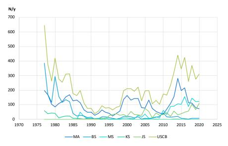
Fig. 4. The annual activity of tremors with energy above 1 MJ (1977– 2020) both for the entire USCB and individual structural sub-units
