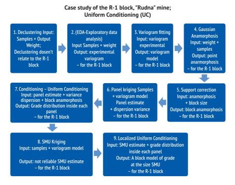
Fig 36. Uniform Conditioning (UC); Workflow; the R-1 block, "Rudna" mine.
