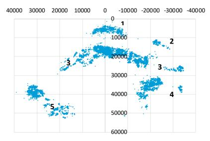
Fig. 1. The distribution of epicenters of strong tremors with energy greater than 100 kJ (1987–2020). The map plotted in the "Sucha Góra" coordinate system. 1) Bytom syncline; 2) Kazimierz syncline; 3) Main anticline; 4) Main syncline; 5) Jejkowice syncline
