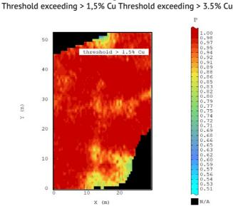
Fig. 34. Raster map of distribution of probability P values of threshold exceeding > 1.5 % Cu; Cu grade in the deposit, the R-3 block, "Rudna" mine
