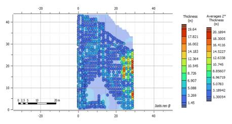
Fig. 18b. Raster map of distribution of estimated averages Z\* of thickness th [m] with sampling points (basemap); the block R-1, "Rudna" mine; the results of ordinary (block) kriging
