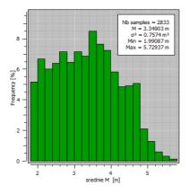
Fig. 31. Histogram of distribution of estimated averages Z<sup>\*</sup> of thickness [m]; the R-3 block, "Rudna" mine; skewness  $g_1 = 0.17$ , quasi-symmetry;  $g_2 = 2.10$ , a platokurtic kurtosis; variation coefficient V = 25.99 %
