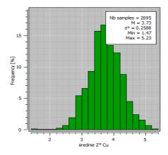
Fig. 30. Histogram of distribution of estimated averages Z\* of Cu grade [%]; the R-3 block, "Rudna" mine; skewness  $g_1 = 0.76$ , week asymmetry;  $g_2 = 5.48$ , a leptokurtic kurtosis; variation coefficient V = 34.46 %
