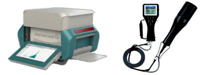
Fig. 5. On the left, a portable EDXRF spectrometer (xenemetrix.com), and on the right, an analyzer for determining basic physicochemical parameters of water by Horiba (horiba.com)
