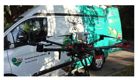
Fig. 7. An example of a measurement set – a drone armed with a portable air analyzer with a built-in air sampling module
