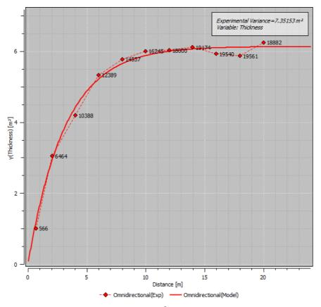
The block R-1, "Rudna" mine. Isotropic variogram of thickness
