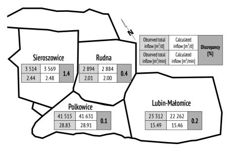
Fig. 3. Summary of the size of groundwater inflows to the workings observed and obtained on the model in  $m^3$ /min
