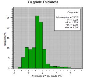
Fig. 19. Histogram of averages Z\* of Cu grade [%] distribution in enclosed Cu ore deposit; the block R-1, "Rudna" mine; skewness  $g_1 = 0.76$ , moderate asymmetry;  $g_2 = 5.48$ , a leptokurtic kurtosis; variation coefficient V = 34.46%
