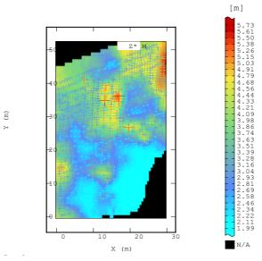
Fig. 29. Raster map of distribution of estimated averages Z\*of the thickness [m]; the R-3 block, "Rudna" mine
