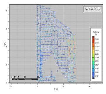
Fig. 6. Basemap with sampling points: thickness [m]; size N=708; distance between samples 15–20 m in the headings; The block R-1, "Rudna" mine
