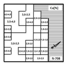
The results of ordinary kriging, applying spherical model of ledge parameters variograms; (elementary grid 100 m × 100 m)
