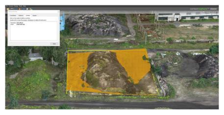
Fig. 6. An example of the use of drone raids equipped with a high-resolution camera. The analysis of photos specialized programs allows you to document the places of sampling or determine the size and location of potential sources of pollution
