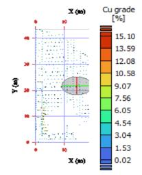
Fig. 11a. VMap of Cu grade [%] in copper ore deposit; R-1 block, "Rudna" mine
