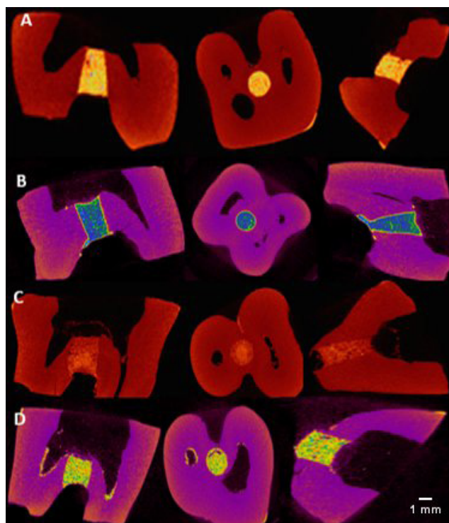
Fig. 3. Samples colored using the DataViewer software to enhance the visibility of the pores
