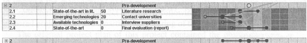
Figure 10. Responsibility of process 2 "Pre-development" is shown as a circle, and collapses to a large dot
