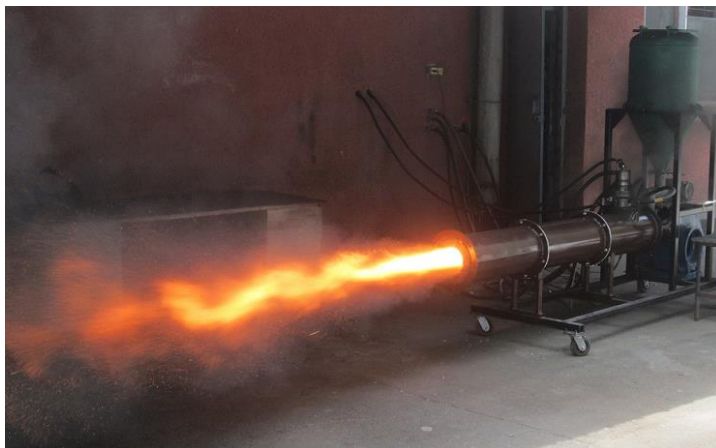
Fig. 1. Bench tests of the plasma fuel system and a flare of high-temperature two-component fuel at the outlet
