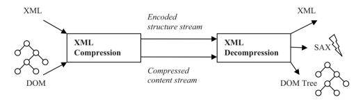
Figure 1. Architecture of the Millau Compression-Decompression System
