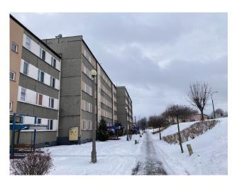
Fig. 1. View of one of the buildings. The thermal modernization so far has been limited to thermal insulation of window strips. The difference in the ground level is also visible (photo by R. Oleksik)
