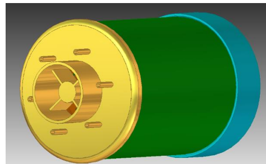
Fig. 2. Three-dimensional model of the reference combustion chamber for numerical investigation
