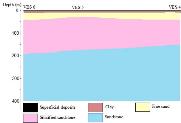
Figure 5. Hydrogeological cross section interpreted from resistivity cross section of profile 1.
