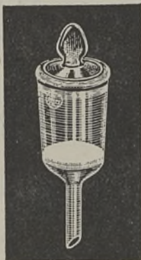
Glass Filter tube with ground-in stopper No. S.F. 5A.
