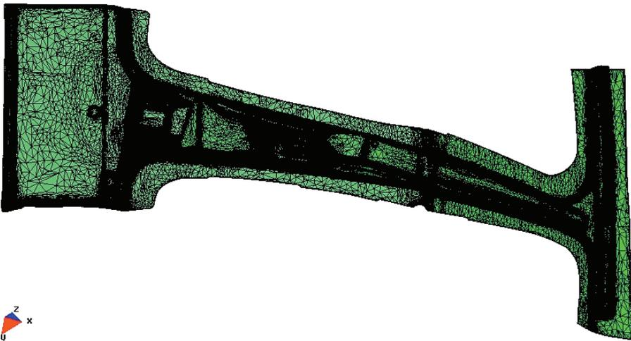
Fig. 2. Geometrical description of final piece (195 079 triangular facets)
