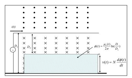
Fig. 2.15: Inductive coupling due to a current above ground.
