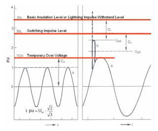
Fig. 5.2: Different types of overvoltage with corresponding insulation levels.
