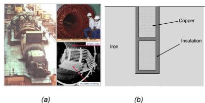
Figure 1.6: (a) Generator, stator windings and (b) detail of the windng insulation in the stator slot
