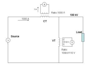
Fig. 1.17: Schematic diagram showing a typical application of current and voltage transformers to a single phase circuit
