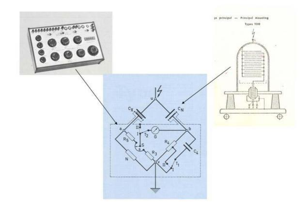
Fig. 4.20: Typical Schering Bridge set-up (Tettex)
