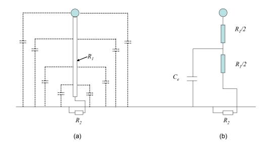
Fig. 4.12: (a) Stray capacitance of a resistive divider and (b) the equivalent circuit
