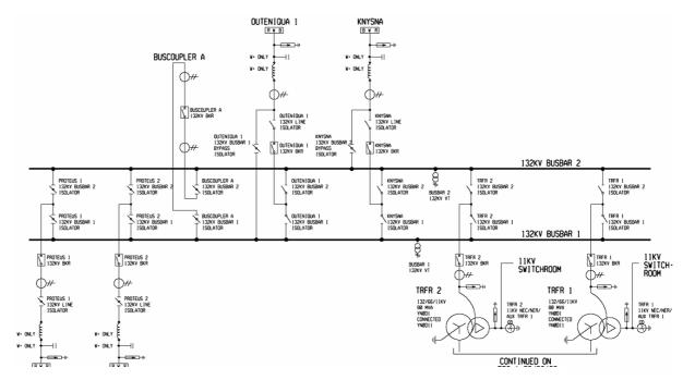
Figure 1.7: Single line diagram of a typical 132 kV substation.
