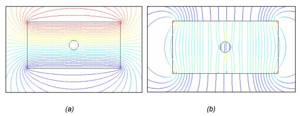
Fig. 2.12: Equipotential lines (a) and field lines (b) for a cylindrical sphere, having a dielectric constant of 6 in an air gap.
