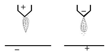
Fig. 3.7: Explanation of the polarity effect of DC flashover of an unsymmetrical arc gap.
