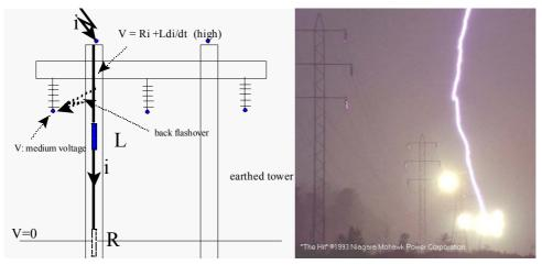
Fig. 5.21: Back flashover to tower due to stroke to tower of shielded line.
