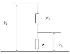
Fig. 4.11: General voltage divider
