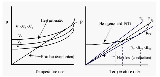
Fig. 3.19: Thermal runaway due to (a) voltage increase and (b) increase in soil thermal resistivity due to the drving out of the soil.
