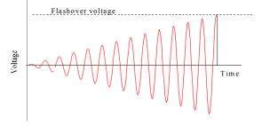
Fig. 4.16: AC flashover with increasing voltage.
