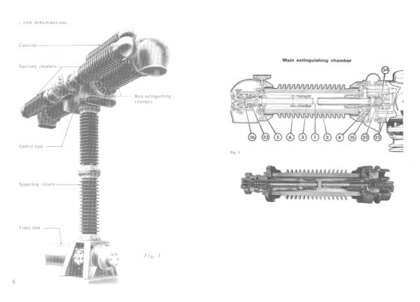
Fig. 1.26: Air Blast Circuit Breakers
