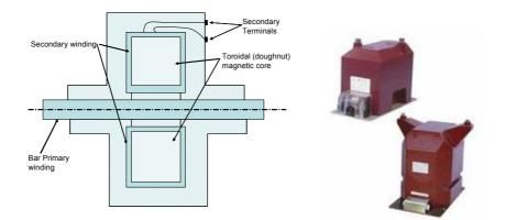
*Fig. 1.19: Epoxy resin encapsulated current transformer for use in medium voltage switchgear*
