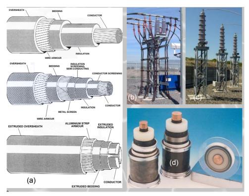
Fig. 1.13: Various types of cable constructions and terminations.
