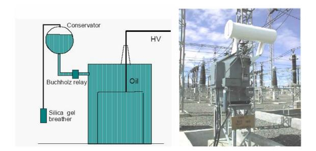
Fig. 3.23: Transformer with conservator and air breather
