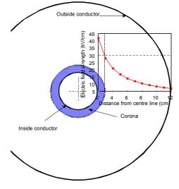
Fig. 3.14: Coaxial cylinders (12 cm/ 2 cm radii) at 150 kV- E > 30 kV/cm in shaded region.
