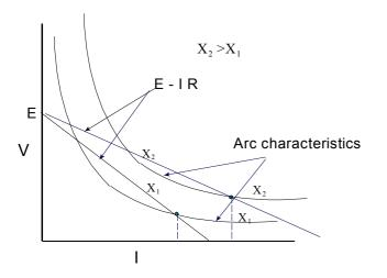
Fig. 3.33: V-I characteristics of polluted layer and dry band arc as dry band widens
