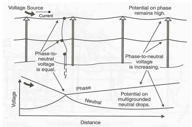
Fig. 6.5: Safety earth on a two-wire line.
