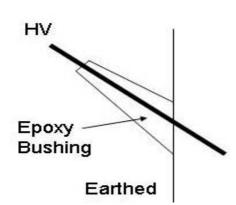
Fig. 3.30: Transformer Bushing
