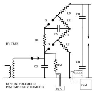
Fig. 4.9: Two-stage impulse generator
