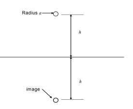
In the case of such a cylinder above ground, the maximum field strength (at the conductor surface) is given by:
