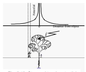
Fig. 5.19: Step and touch potential due to lightning.
