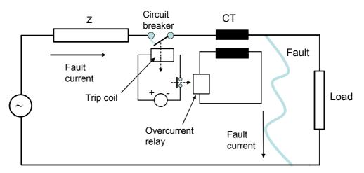
*Fig. 1.25: Schematic presentation of the interruption of fault current by a circuit breaker and associated protection relays.*
