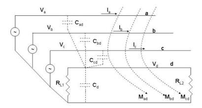
Fig. 6.4: Electromagnetic induction
