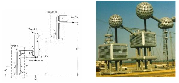
Fig. 4.3: Cascade connected test transformers
