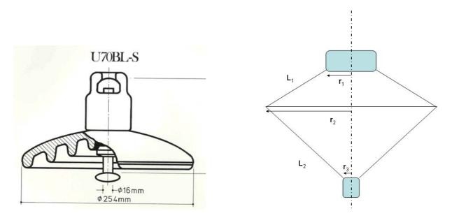
Fig. 3.35: (a) Typical cap and pin insulator. (b) Simplified model of Insulator shown in Fig. 3.35 (a) and using this data as inputs to a numeric integration procedure.
