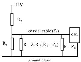
Fig. 4.13: Resistive impulse divider
