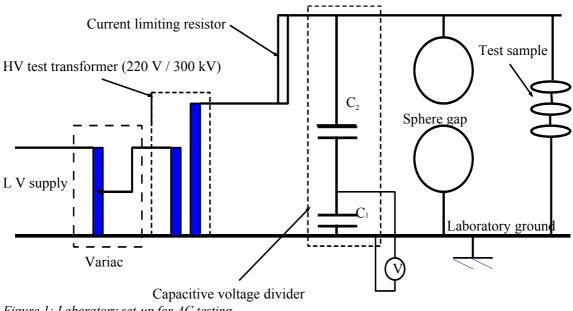
Figure 1: Laboratory set-up for AC testing
