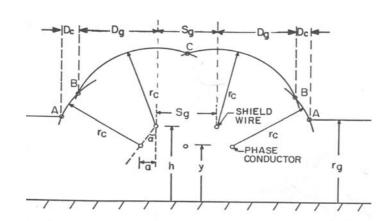
Fig. 5. 17: The geometrical model for line lightning protection.
