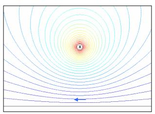
Fig. 2.14: Magnetic Field lines of a conductor above ground.
