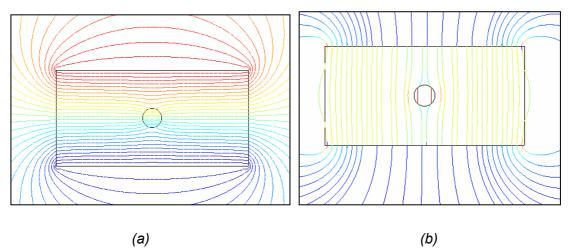
Fig. 2.11: Equipotential lines (a) and field lines (b) for a cylindrical void in a dielectric, having a dielectric constant of 6
