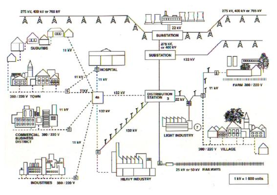
Fig. 1.1: Schematic representation of a power network
