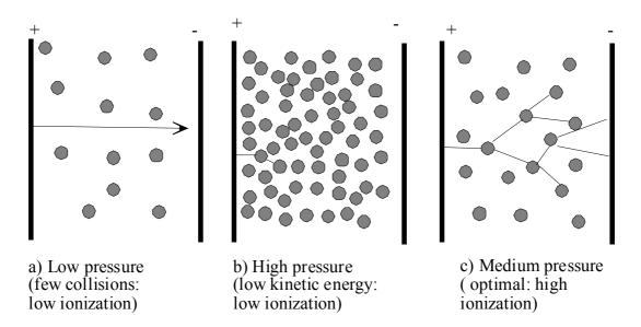
Fig. 3.6: Ionisation by electron collision with gas atoms
