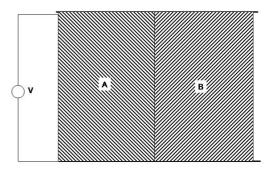
Fig. 3.24: Parallel Insulating materials
