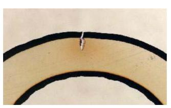
Fig. 3.20: Typical samples of treeing in solid insulation
