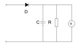
Fig. 4.15: Typical AC peak voltmeter circuit
