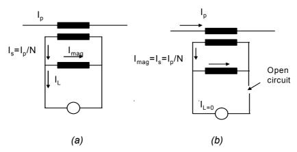
*Fig. 1.20: Equivalent circuit of current transformer (a) normal operation and (b) with opencircuited secondary.*
