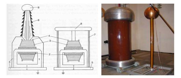
Fig. 4.2: Typical designs of AC test transformers
