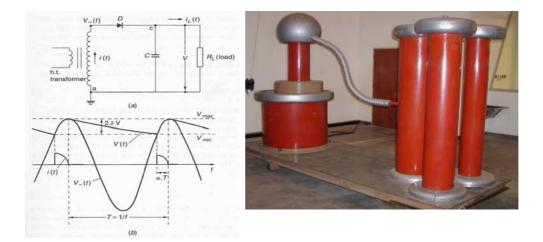
Fig. 4.6: Typical waveforms and a typical doubling circuit DC test source
