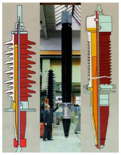
Fig. 1.15: Examples of typical graded bushings
