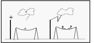
Fig. 5.20: Induced overvoltages due to nearby lightning stroke
