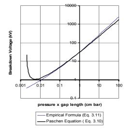
Fig. 3.5: The Paschen curve for air
