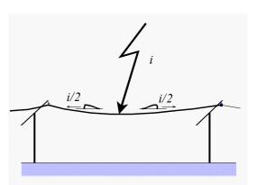
Fig. 5.18: Direct lightning stroke to a line
