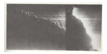
Fig. 5.11: Streak photograph of lightning development
