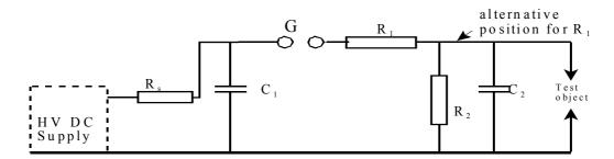
Fig. 4.8: Single stage impulse generator
