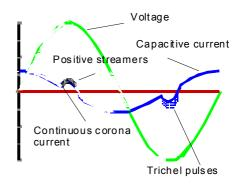
Fig. 3.15: AC Corona voltage and current wave forms
