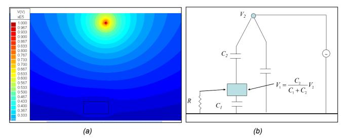
Fig. 2.13: Electrostatic induction (a) and capacitive equivalent circuit (b).
