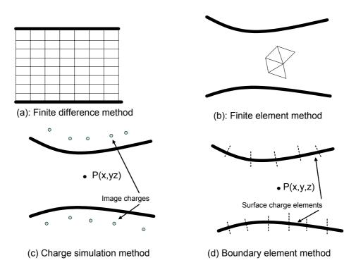
Fig. 2.17: Principal methods of field simulation
