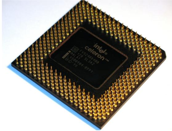
Figure 6.6 The downside of Intel Celeron microprocessor in a PGA packaging
