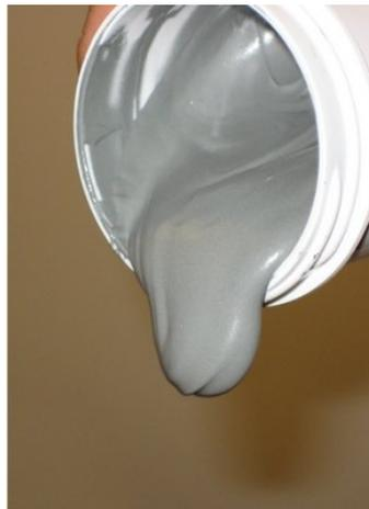
Figure 7.2 Solder alloy paste [25]
