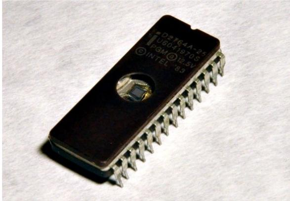
Figure 6.8 Ceramic Dual In-line Package
