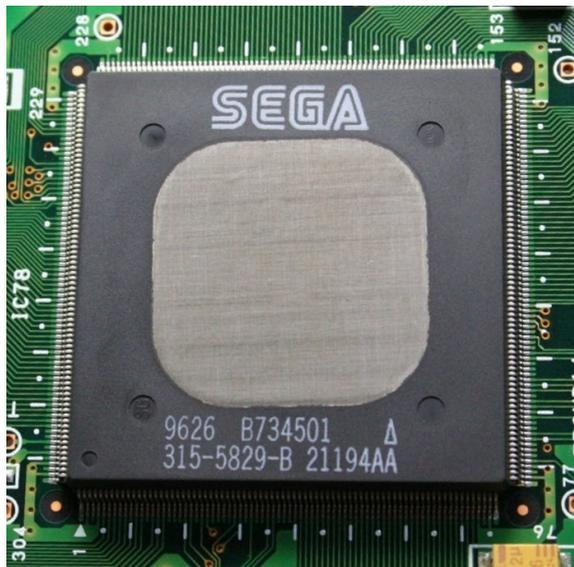
Figure 6.20 304-pin QFP chip produced by SEGA (Courtesy of Wikimedia Commons)
