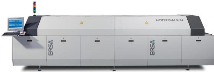
Figure 8.10 ERSA reflow oven for reflow soldering [32]
