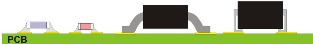
Figure 8.2 One sided PCB with SMD components prepared for reflow soldering
