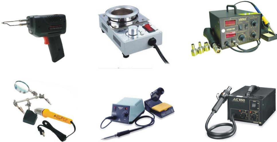
Figure 8.6 Basic equipment for manual soldering (Courtesy of producers, source: Google Image)
